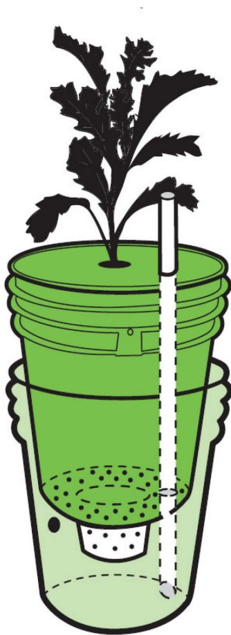
DIAGRAM OF A SELF-WATERING CONTAINER
